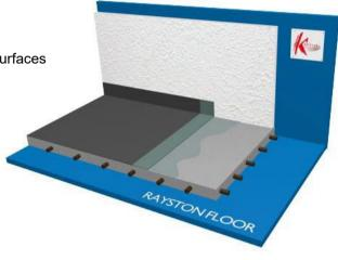
BASE: Concrete, >28-day curing time, moisture level <4%, no rising damp, strength <1.5N/mm2, Temp. > 10°C, without any contamination, grease, dust or open pores.
