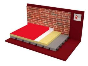
Approximate thickness of the system: 1-2-3 cm (depending on the density and amount of foam applied).
